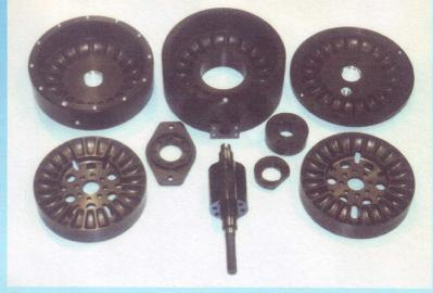
Simple and rugged characterizes the Island City DHG construction.. Monolithic CNC machined components are TYPE III anodized per MILSPEC for corrosion and erosion protect. Hard housing surface finish (85 Rockwell) is approved for potable water and food applications. Operating temperature range to 220 deg F [xxx deg C] with higher operating temperature available upon application.
