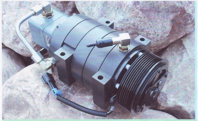
The ISLAND CITY Dynamic-Heat-Generator is a MECHANICALLY DRIVEN fluid heater. Only rotary shaft input is required to heat large fluid volumes rapidly and efficiently without a heat exchanger. ORIGINALLY developed to heat and maintain diesel engine temperature in arctic conditions the DHG is adaptable to many heating applications. Driven from engine PTO, electric motor, hydraulic drive or belt the DHG has one moving functional component requiring no regular service or consumables.
